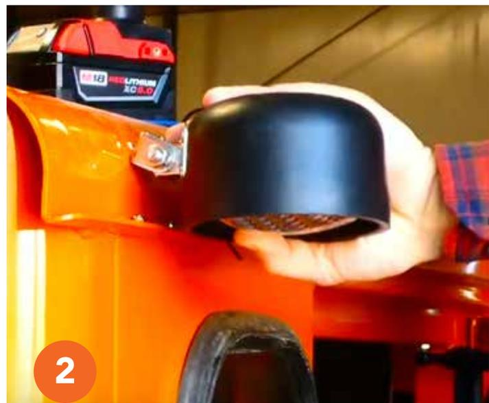
3. Push the bushing into the available hole next to the light. Then take the wire, make sure it's stripped, and push it through the hole.
