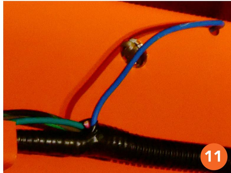
12. Just to the top right of the harness, you'll see a little metal button, just push it out and then slip the blue wire in the open hole.
